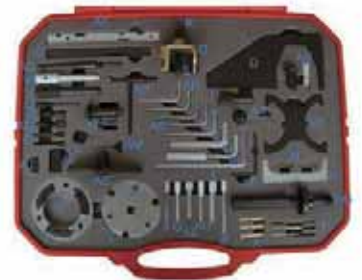
TATHT308 Engine Timing Tool Set - FORD 1.25L, 1.4L, 1.6L, 1.8L, 2.0L & 2.4L
