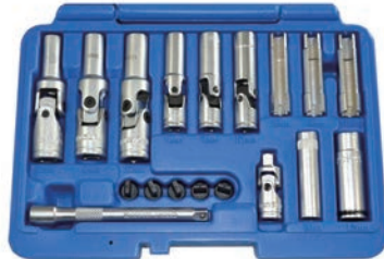
TATPC826 Special Thin Glow Plug Removal Socket Set 18pcs
