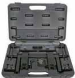
TATHT298 Engine Timing Tool Set For Professional Engine Repair - BMW N51, N52
